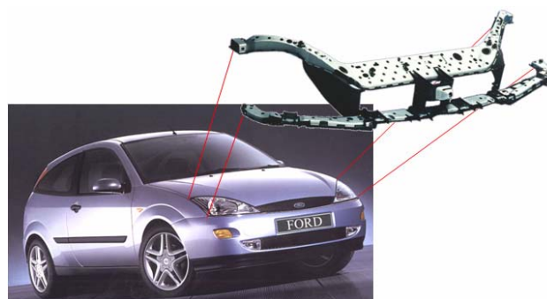
Figure 2 As a component of the car body, the GOR of the Ford Focus helps in all driving and crash situations to stabilize the front of the vehicle.
