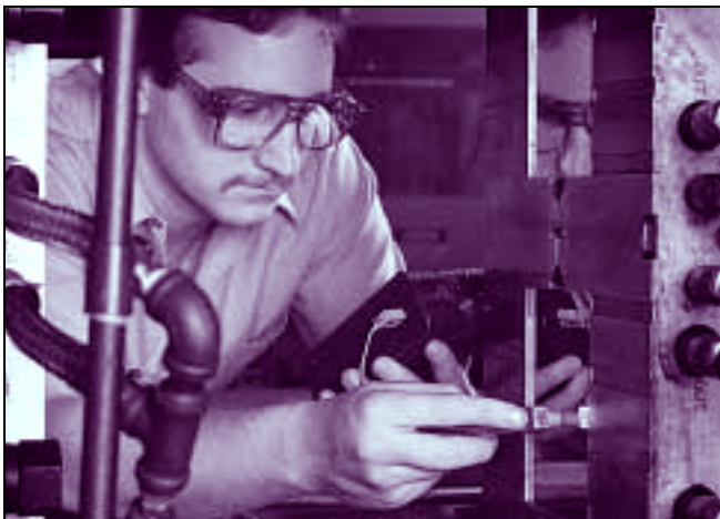
Figure 16 Measuring Mold Surface Temperature During the Injection Molding Cycle
