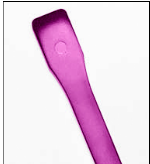
Figure 46 Poor Surface Finish/ Lack of Gloss
