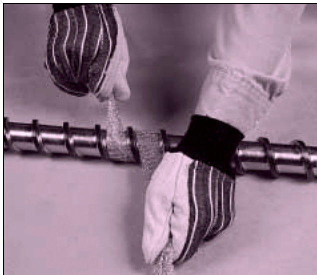
Figure 25 Mechanical Cleaning of the Screw
