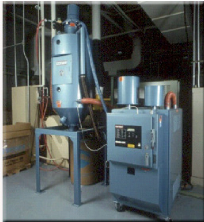
Figure 12 Typical Desiccant Dehumidifying Hopper Dryer System
