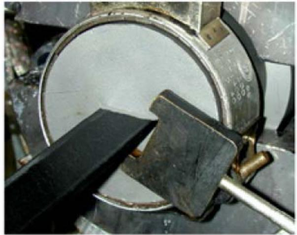
Figure 5 Fork sensor located between the die and the calibration unit
