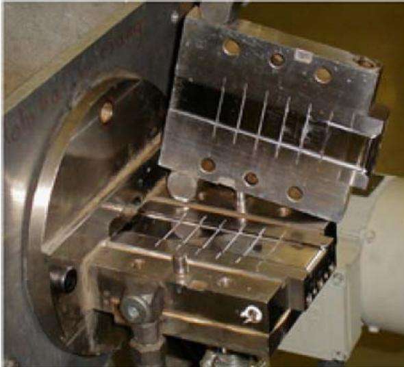
Figure 4 Calibration unit in open position
