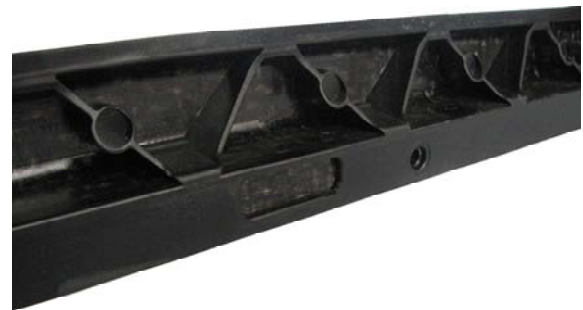
Figure 2 Detail of the nylon composite sheet reinforcement for the lower beam
