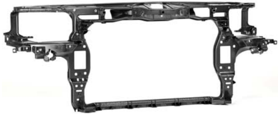
Figure 1 The lower beam of the front end features a U-shaped profile made of composite plastic sheet.
