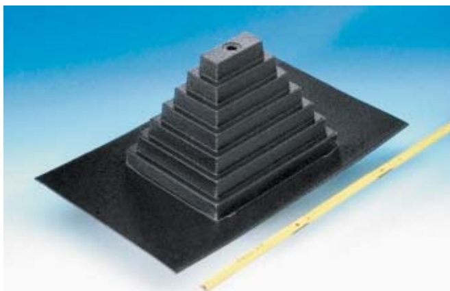
Figure 6: Step pyramid, stretching ratio 1:2.4
