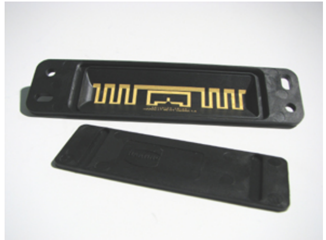
Figure 3 Three-dimensional antenna structure produced using LDS technology
