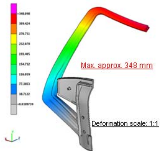
Fig. 2 Simulation of the deformation under static loading
