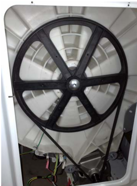
Figure 1 Belt pulley for a washing machine drum
