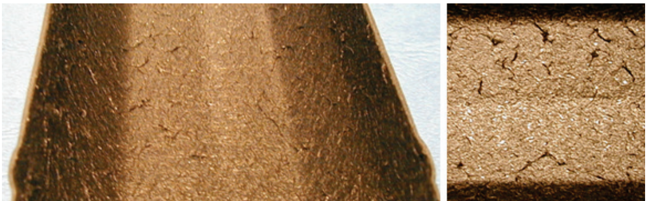
Fig. 3 Defects due to "beard" formation
