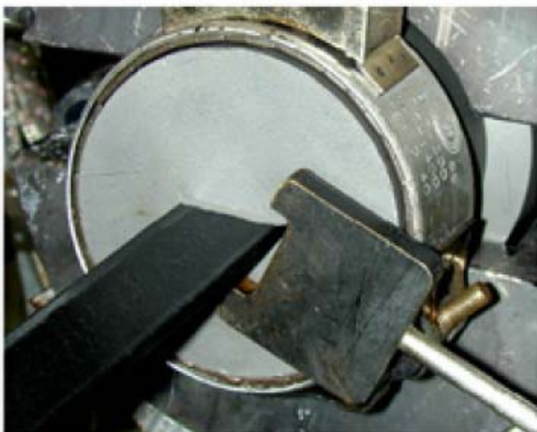
Figure 5 Fork sensor located between the die and the calibration unit
